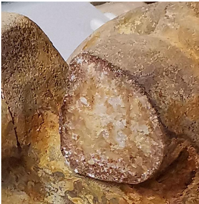
Fig. 8. Ingrown oxidation (brown) into the marble core, indicating a long-term process. Heerlen, coll. B. Blok.
